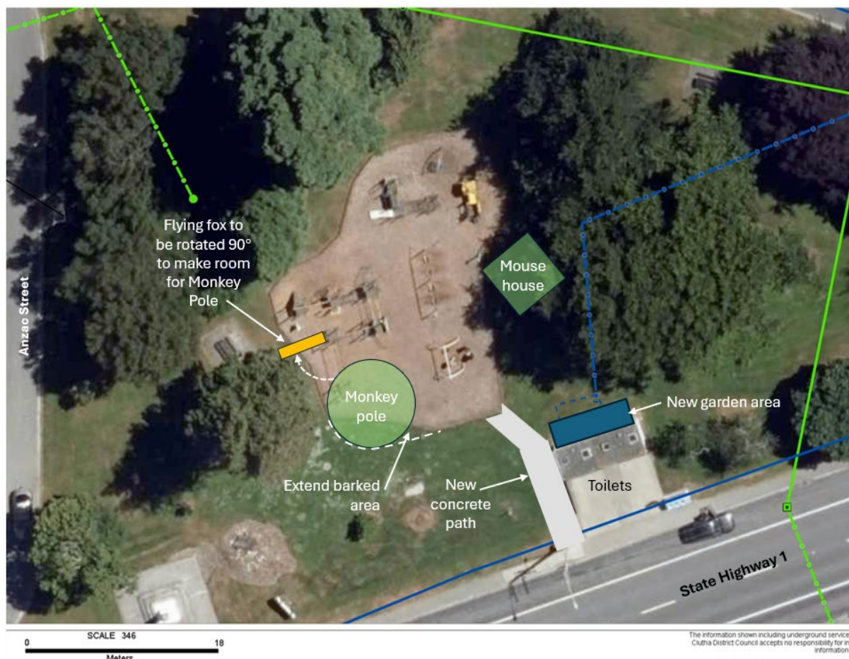
Figure 4 Design plans for the Clinton playground upgrade. Blue & green lines are water pipes.
