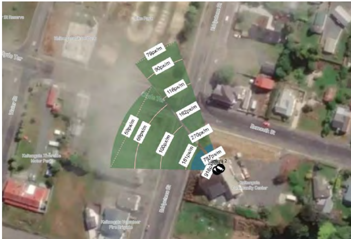
Figure 1 Plan view of CCTV coverage
